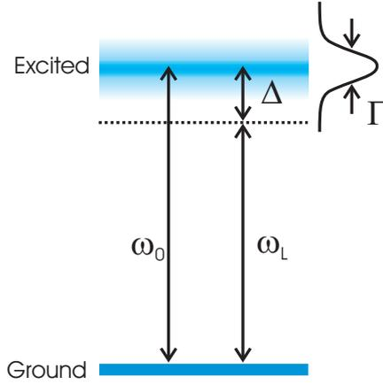
**Figure 2.1:** The two-level model showing the atomic transition angular frequency  $\omega_0$ , the laser light's angular frequency  $\omega_L$ , the detuning  $\Delta$  and the natural line width of the excited state  $\Gamma$ .
