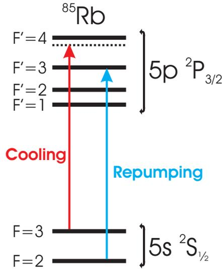
**Figure 2.5:** The energy level diagram for  $^{85}\text{Rb}$ . The transition frequencies for the cooling and repumping lasers are also shown. This figure should be contrasted with the simpler two-level model in Figure 2.1. The level spacings are given in Appendix D.
