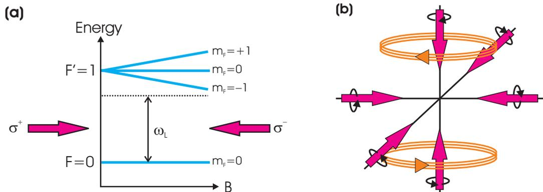
**Figure 2.4:** Plot (a): The principle of a magneto-optical trap is demonstrated for the  $F = 0 \rightarrow F' = 1$  transition. An atom that has moved away from the trap centre is more likely to absorb a photon from the beam pushing it back. This results in a harmonic force. Plot (b): The simplest design for a 3D magneto-optical trap made from six circularly polarised laser beams. The anti-Helmholtz coils created a quadrupole magnetic field.
