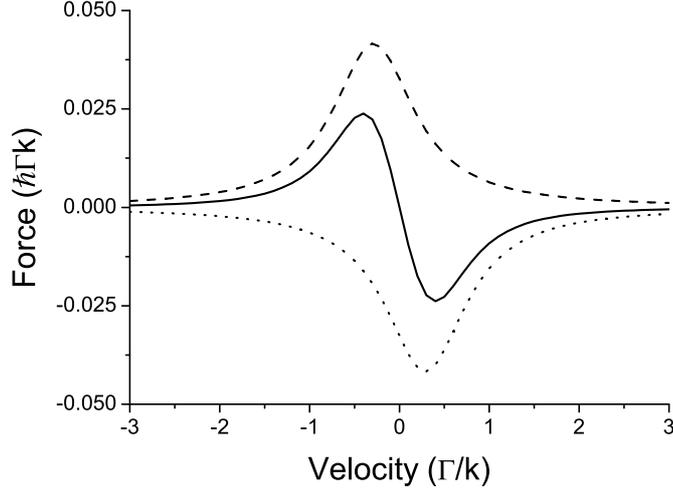
**Figure 2.3:** The combined force of two counter propagating red-detuned laser beams is plotted against velocity. The dashed line is  $F_+$ , the dotted line is  $F_-$ , and the solid line is the total force  $F_{\text{tot}}$ . The parameters used to produce the plot were  $I/I_{\text{sat}} = 0.1$  and  $\Delta/\Gamma = -1/\sqrt{12}$ .
